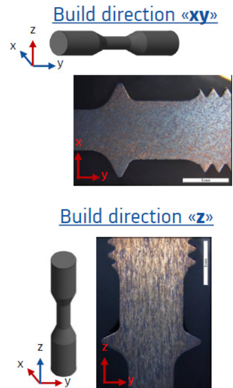
Figure 6: Tensile specimens produced in different orientations by the laser powder bed fusion AM process.
