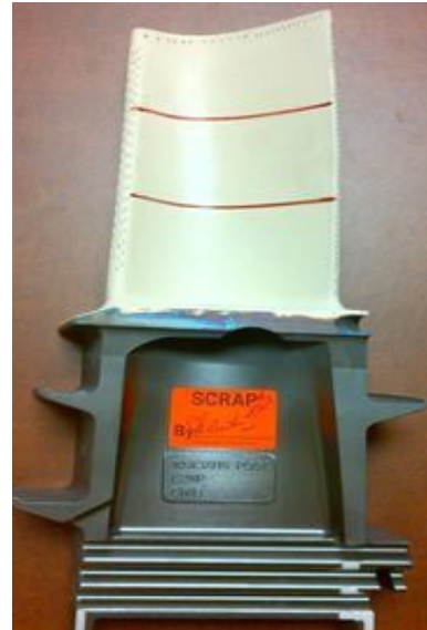
Figure 2: Scrapped Fr7FA.03, stage 1 bucket after 3 engine service (hot gas path) intervals
