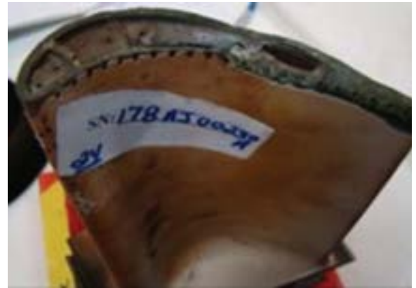
FIGURE 1: A Fr7FA.02, stage 1 bucket after 2 service intervals
