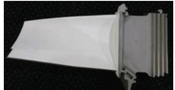
FIGURE 1: Siemens W501F, row 2 blade that was repaired via HIP Rejuvenation
