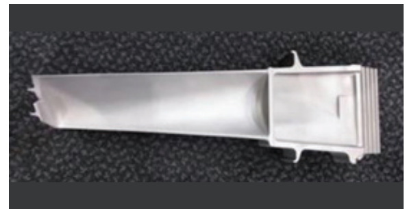
FIGURE 1: Fr7B, 2nd stage bucket that operated for 3 service intervals.
