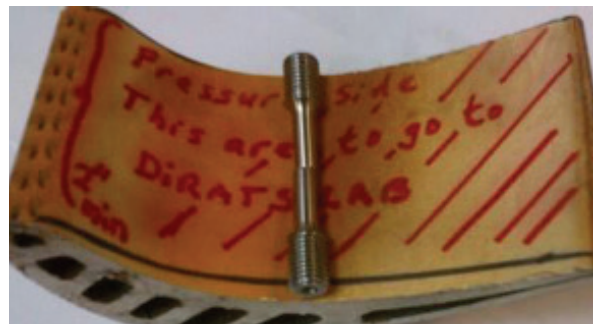
Figure 4: Schematic of removing tensile and stress rupture specimen from the airfoils.
