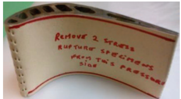
Figure 3: Section of the airfoil removed by water-jet cutting for destructive analysis
